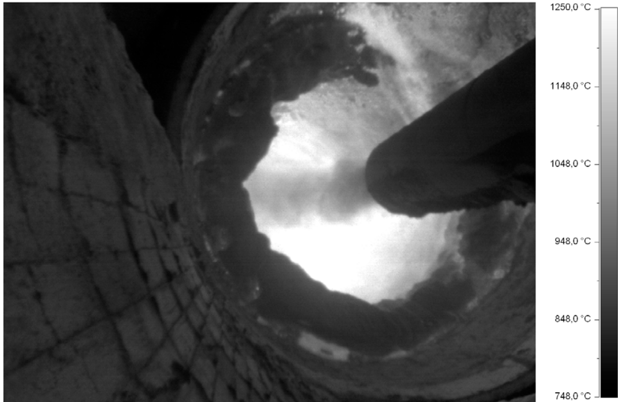
Fig. 10: IR-image taken from the kiln hood, burner located on the right.
